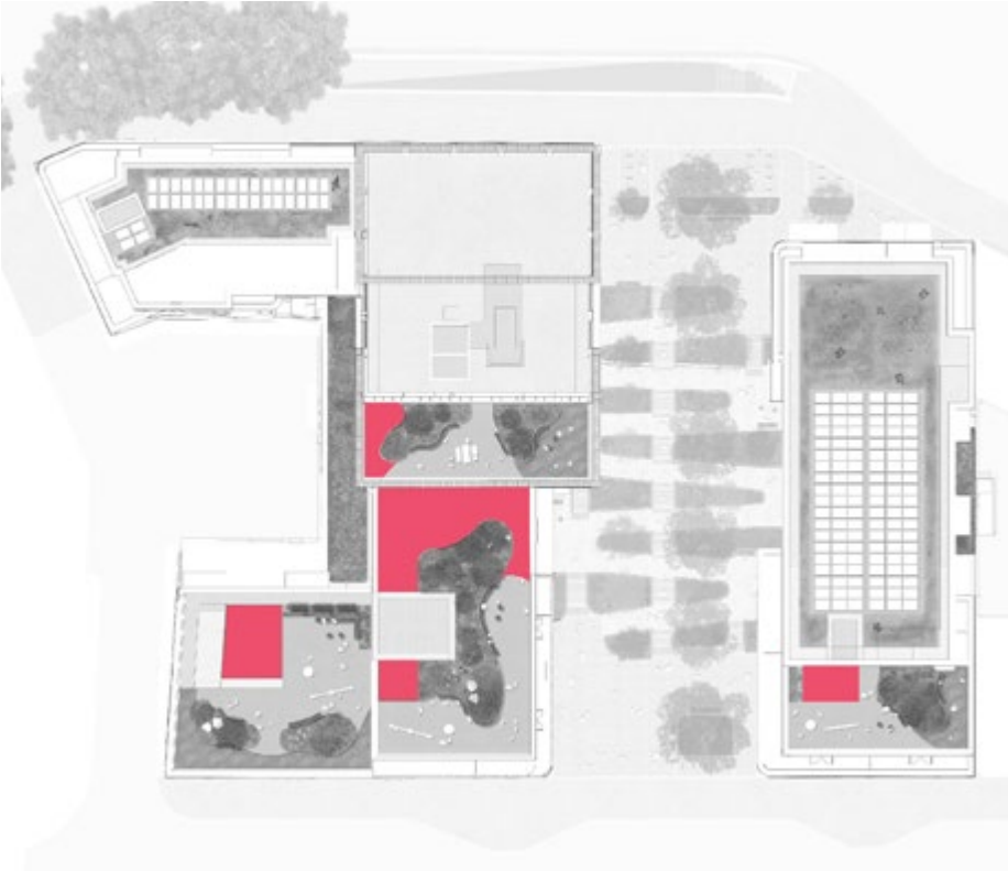
Location highlighted - Decking to amenity roofs
