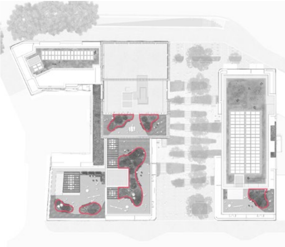
Location highlighted - raised metal edge to amenity roof planters
